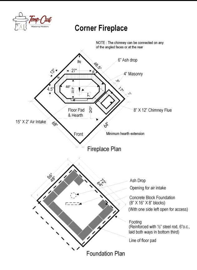
NOTE: If back-up block is required around the chimney, (eg. for stone facings), footing, foundation and pad dimensions will require suitable adjustment.
