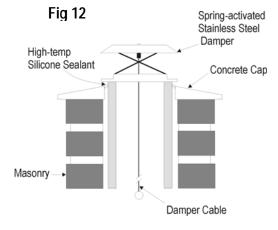
chimney adapter is installed on top of the last clay flue tile and an 8" (200mm) diameter factory-built stainless steel chimney continues from this point. This "hybrid" chimney allows a roof-top damper to be installed at the top of the factory-built chimney.
