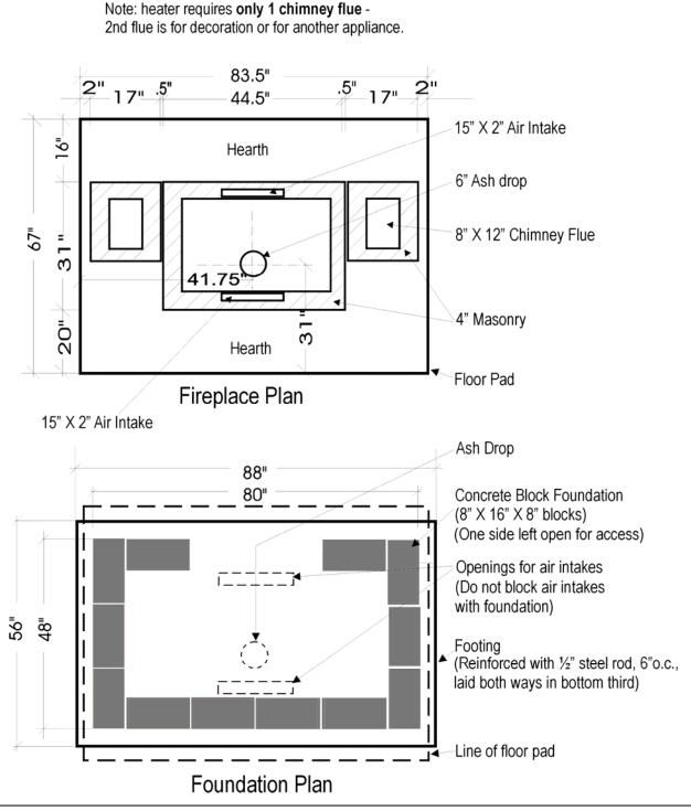
NOTE: If back-up block is required around the chimney, (eg. for stone facings), footing, foundation and pad dimensions will require suitable adjustment.
