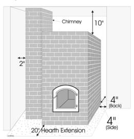
NOTE: a combustible wall with non-combustible material applied directly to it without an intervening air space *IS STILL A COMBUSTIBLE WALL FOR PURPOSES OF CLEARANCES*. If clearances must be reduced, a simple method is to build a wall behind the fireplace, in the area of concern, constructed of "cement board" (a 1/2" [12.5mm] cement sheet) installed on metal studs. This wall section must extend 8" (200mm) beyond the sides of the fireplace.
