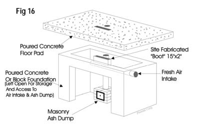
smooth duct is built into the top course of foundation blocks, which will feed necessary air into a 15" x 2" (380mm x 50mm) hole located in the floor pad, directly in front of the unfinished core. The duct is vented to the outside wall under the floor joists and can be equipped with an optional electrically operated damper.
