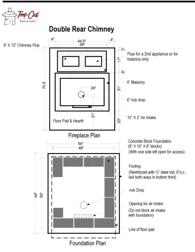
NOTE: If back-up block is required around the chimney, (eg. for stone facings), footing, foundation and pad dimensions will require suitable adjustment.
